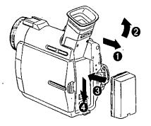
Slide the Viewfinder backward to its fully extended position and then tilt it upward.
