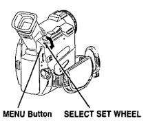
Press MENU to display the camera mode menu in the EVF or the LCD monitor.
