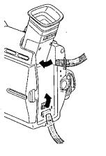
Thread the strap ends through the Strap Attachment Rings.
