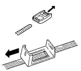
Remove the buckle from one end of the strap.
