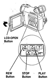
Press the LCD-OPEN Button to unlock the LCD monitor and swing it open.
